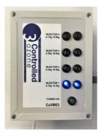
**Co Control Panel** Dimensions: 250 x 155 x 105 mm 8x LED Indicator Lamps Electronic Air Pressure Sensor 1x 5 pin Monitor Output Socket 3x 3 Pin Co Output Socket
